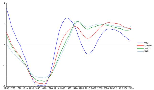
Example spectra: spectra of dried soil samples with 2.2 sensor range (1750 to 2150 nm) after SNV pretreatment. \*Standard normal variate (SNV) is an effective pre-treatment method for baseline correction.
